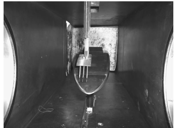
Fig. 4 Model in the test section of T-313 for pitot rake measurements.
